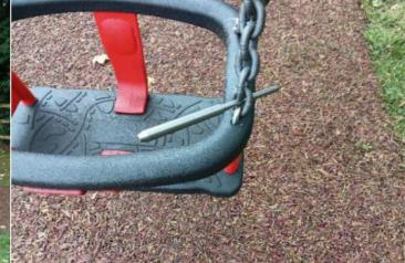
**Finding:** The chain openings are in excess of the 8.6mm as **Action:** Monitor - No action given the risk assessment recommended by BS EN 1176
