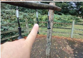
**Finding:** The handgrip has worn and wire strands are exposed
