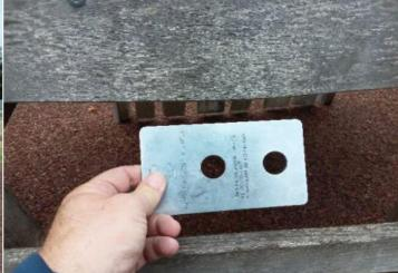
**Finding:** The item fails to meet the requirements of BS EN 1176 Part 1 4.2.7.2 for head and neck entrapment between the ladder rung and platform
